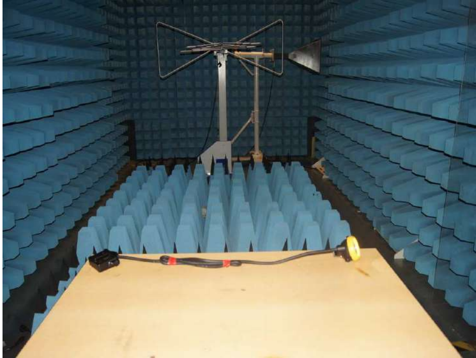
Photograph 3: Set-up for Radio-Frequency Electromagnetic Field (RS)
