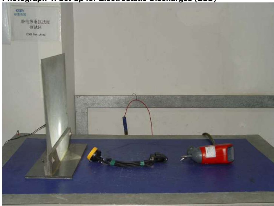
Photograph 4: Set-up for Electrostatic Discharges (ESD)
